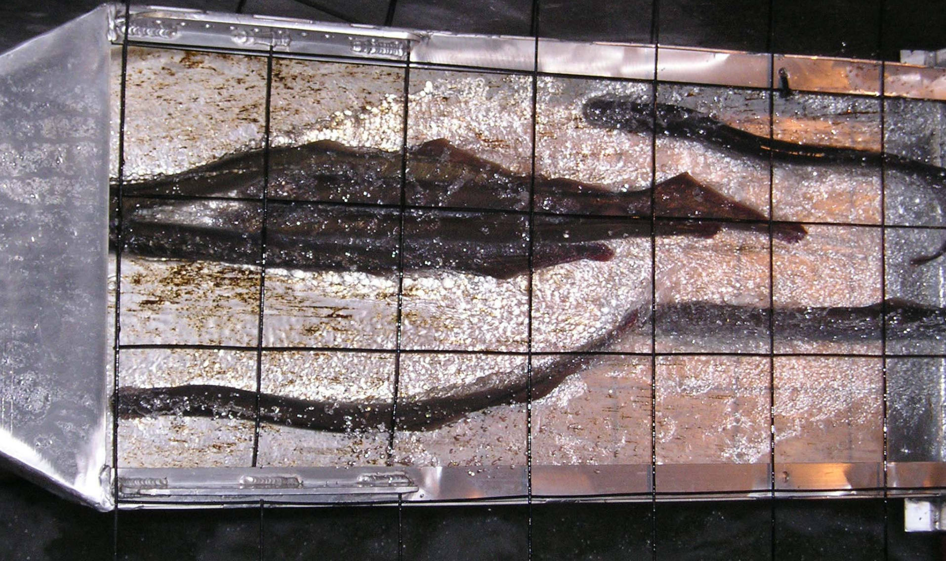
Lamprey Passage Structure (LPS)
