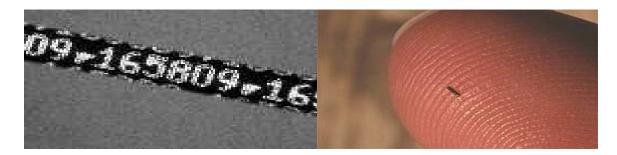
**Figure 1.A.1.1.** A decimal coded wire tag (0.25 mm x 1.1 mm; Northwest Marine Technology photos)
