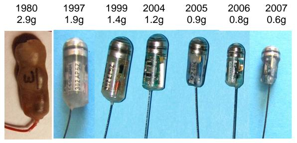
Figure 4.A.3.1. Development of radio tag transmitters over time.
