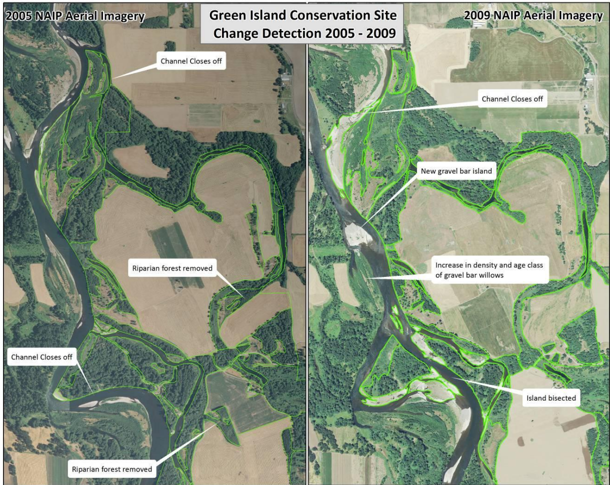
Figure 3. Change detection of riparian forests and hydrology changes using aerial imagery and field visits at Green Island.
